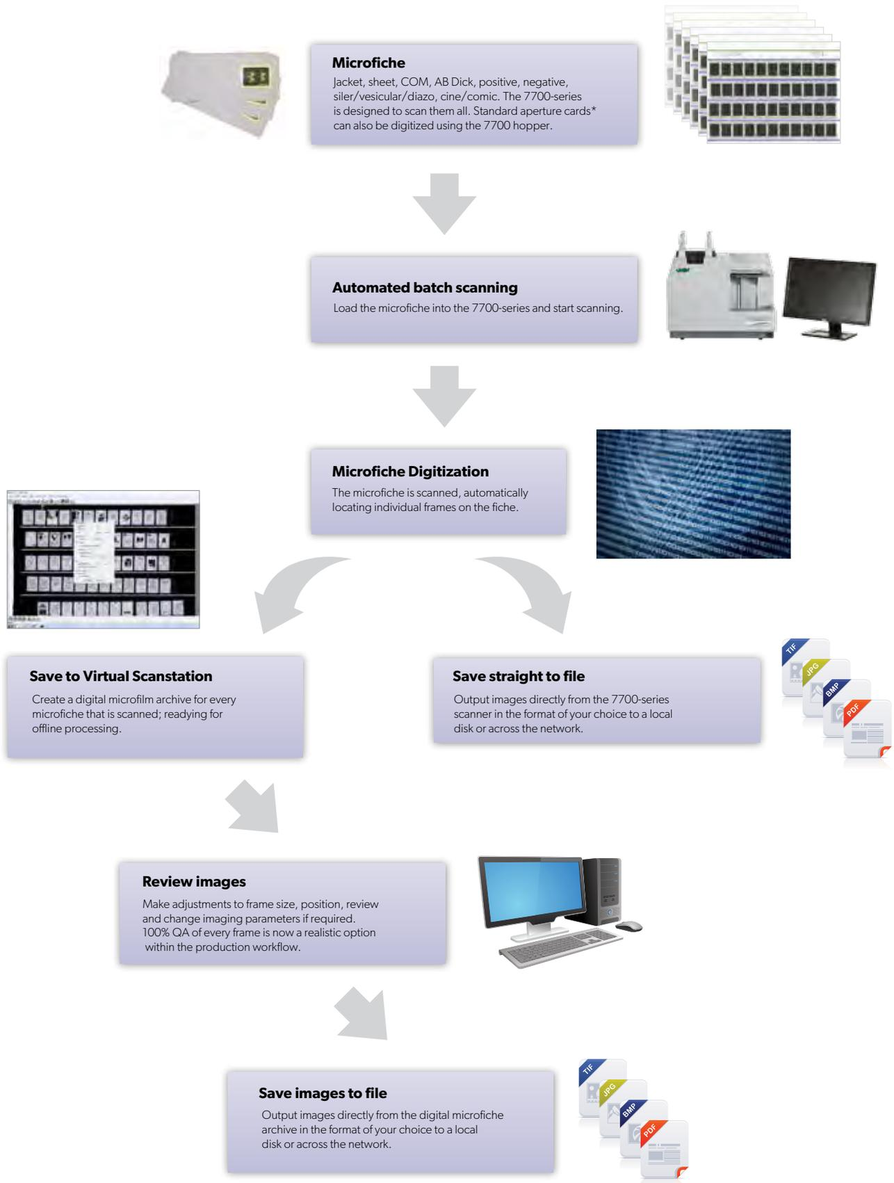
\*The 7700 scans images from the aperture window, but does not read Hollerith code. If Hollerith reading is required, consider the Wicks and Wilson C400 aperture card scanner.
